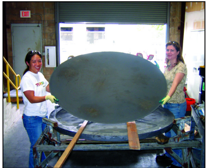
▲ Workers display a silicon-carbide “face sheet” used in the production of large, industrial mirrors made by Trex Advanced Materials.
