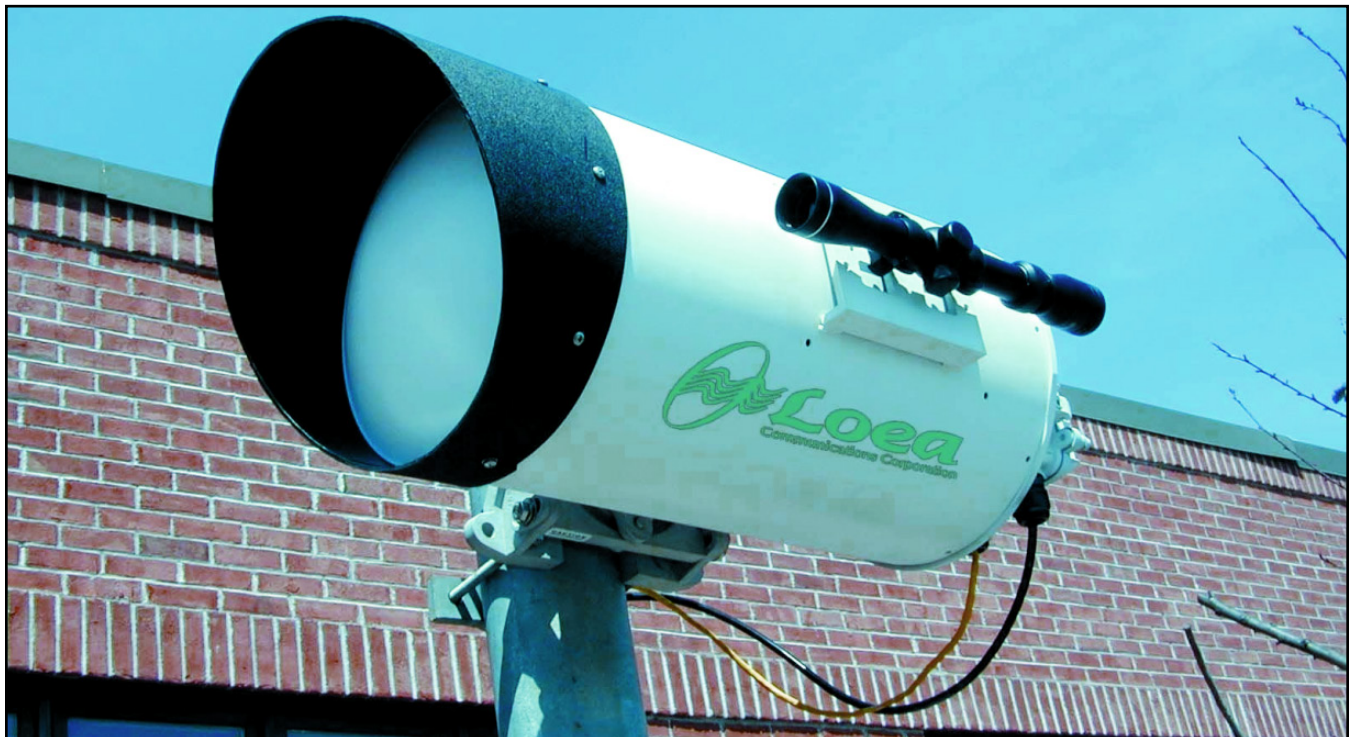
▲ The L1000 system from Loea Corporation, a subsidiary of MDA-funded Trex Enterprises, offers a high-bandwidth, high-speed, wireless alternative to fiber-optic communications.
